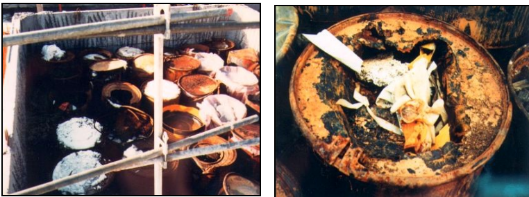
Damaged and leaking waste barrels inside CSM
