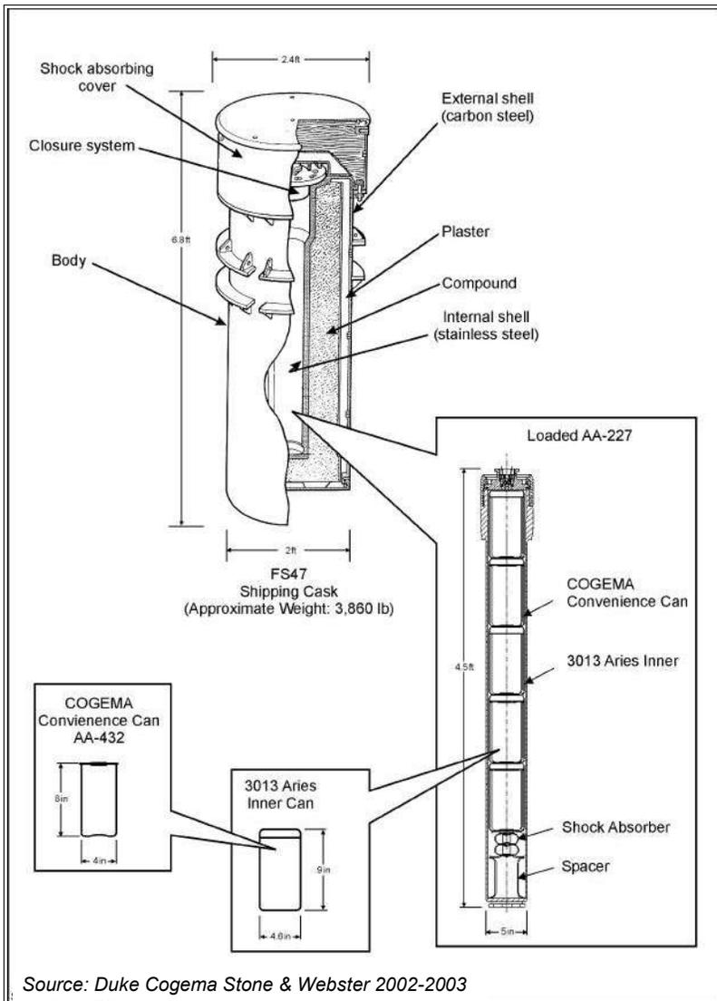
**Figure 1. Cross Section of FS 47 Cask**
