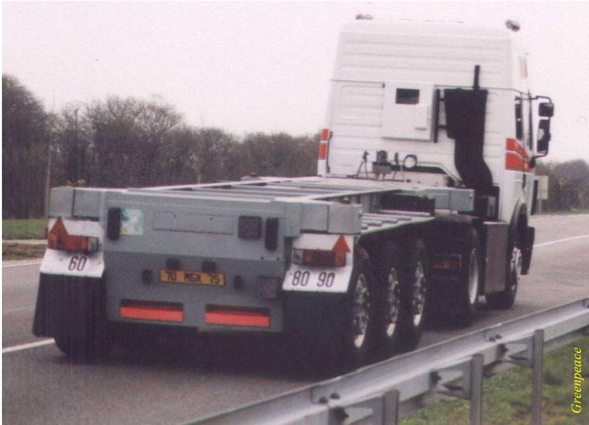
**Photo 3: French plutonium transport trailer without ISO container**
